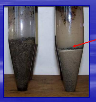
Small spheres of oil (test done below the TIAC)
